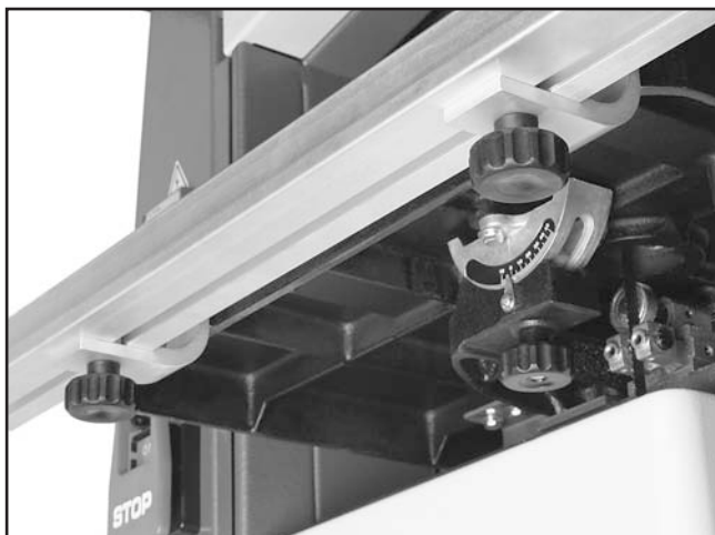
Figure 10. Fastening front fence rail.
